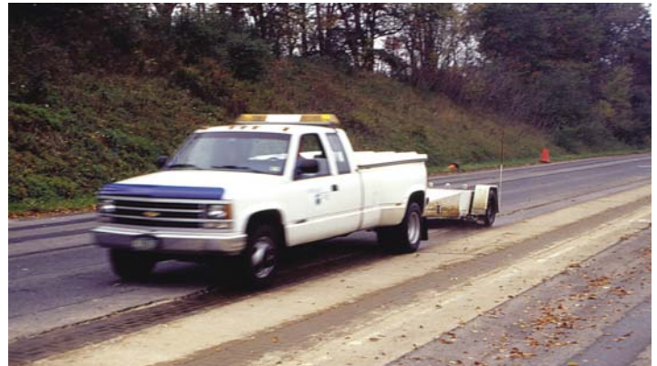
Figure 3. Skid resistance measured on concrete pavers at Pennsylvania Transportation Institute in 1997 according to ASTM E 274 that includes a trailer and tire that locks or skids over a wet surface.
