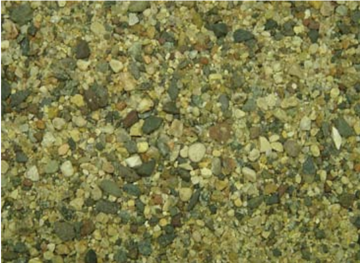
Figure 4. Example of sand from the ICPI bedding sand test program with a total combined percentage of sub-angular and sub-rounded particles equal to 65% according to ASTM D 2488
