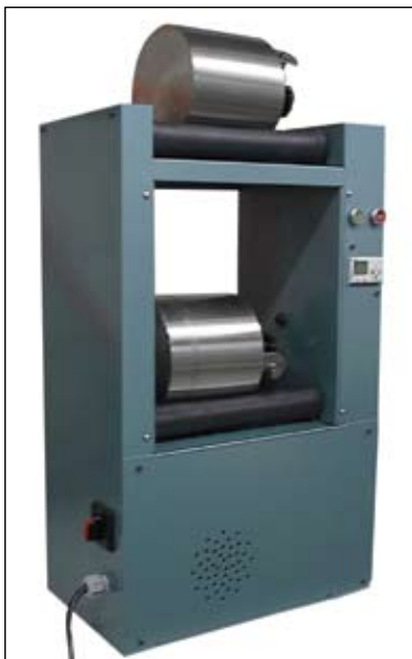
Figure 1. The Micro-Deval test apparatus shows steel jar mills which are rotated while containing sand samples mixed with water. Photo courtesy of Geneq, Inc.
