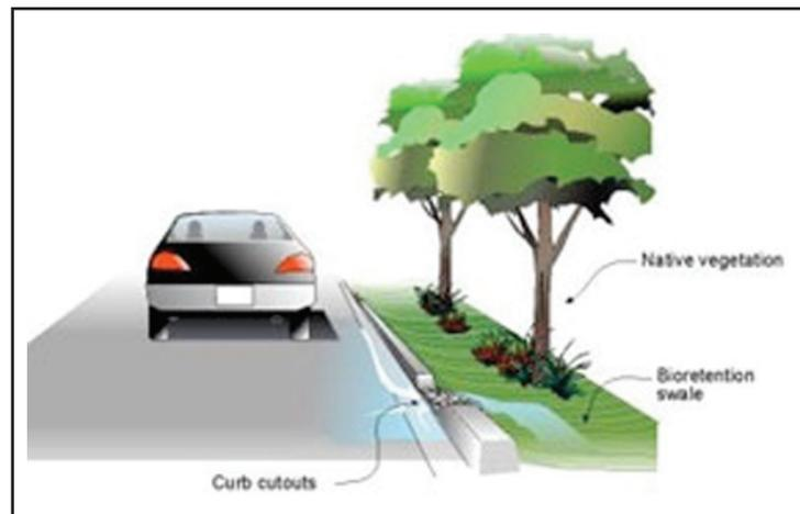
*Figure 2.5a Curb Cuts Schematic*
