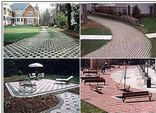
**Figure 3.3.8-4 Examples of Porous Paver Surfaces**
