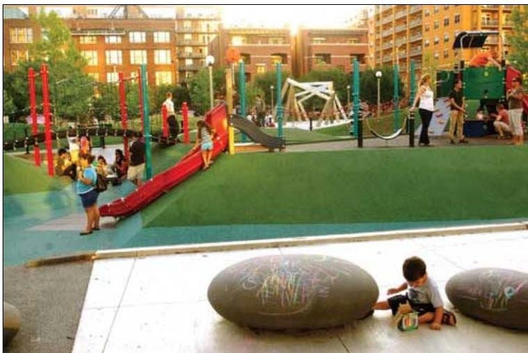
**Mounds formed from recycled rubber surfacing (Total Surfaces) are connected**
