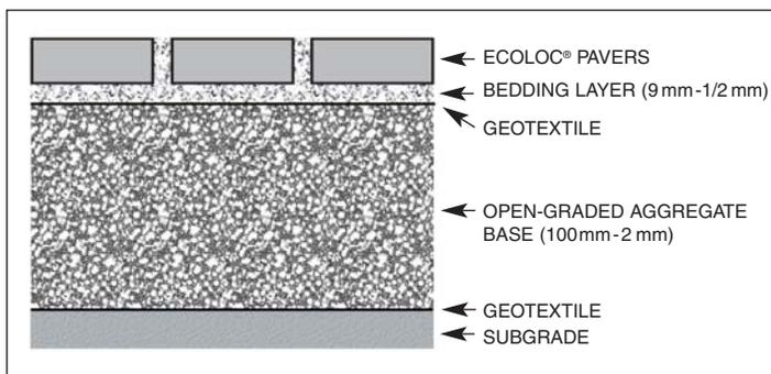
In the pavement cross-sections that utilize the center asphalt travel lane in conjunction with the Ecoloc® parking lanes, the drainage base layer extends
