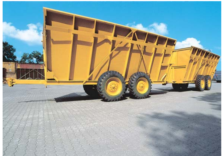
Tractor-pulled cane trailers are used to transport raw cane to the facility
