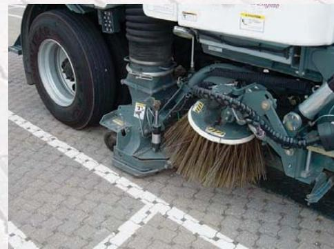
uncleaned area. After cleaning, fresh aggregate material was swept into the joints and drainage voids and the pavement surface was restored to its original condition. This demonstration
