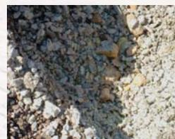
Once the selected Ecoloc pavers were removed, there was no visible sediment on the bedding aggregate or the No. 57 stone base material. This clearly demonstrates the ability of the joint and drainage void aggregate to trap sediment at the surface.
