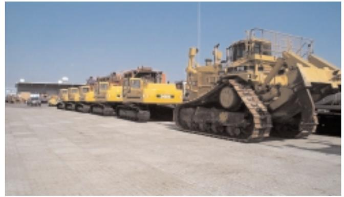
High abrasion resistance to steel tracked equipment is why over a half a million square feet (over 50,000 m<sup>2</sup>) of concrete pavers were used at Dundalk in the Port of Baltimore.
