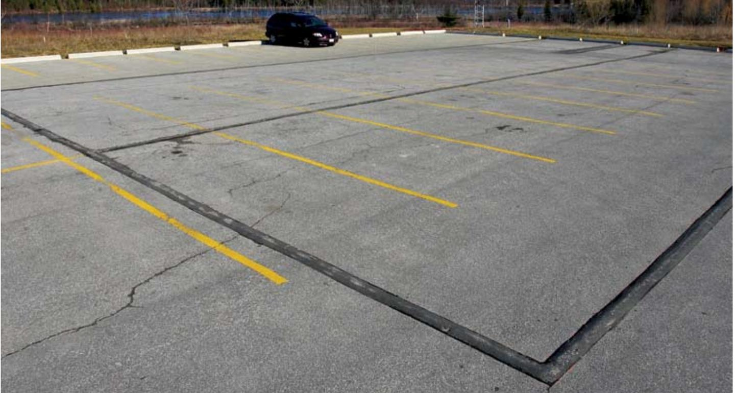
Figure 2. The test area is subdivided in two asphalt areas and one PICP area in the background. The asphalt curbs separate the runoff from each area.
