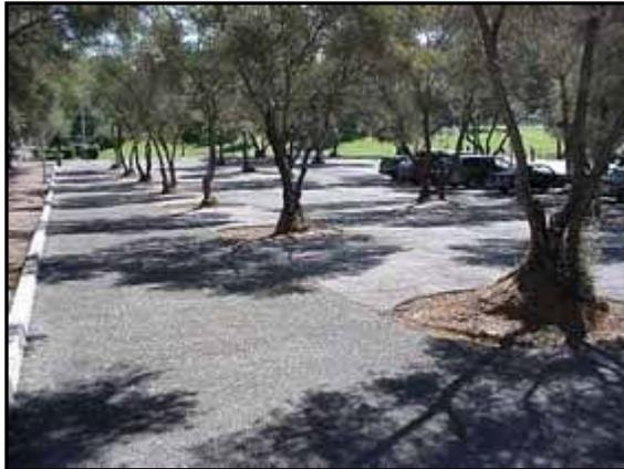
**Description:** Infiltration practices that are alternatives to traditional asphalt and concrete surfaces. Stormwater runoff is infiltrated into the ground through a permeable layer of pavement or other stabilized permeable surface.
