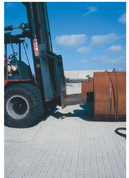
*A Taylor TEC-450L transports a roll of coiled sheet steel weighing over 37,000 lb*
