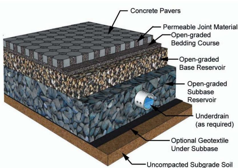
Figure 1 - Permeable Pavement Cross Section
